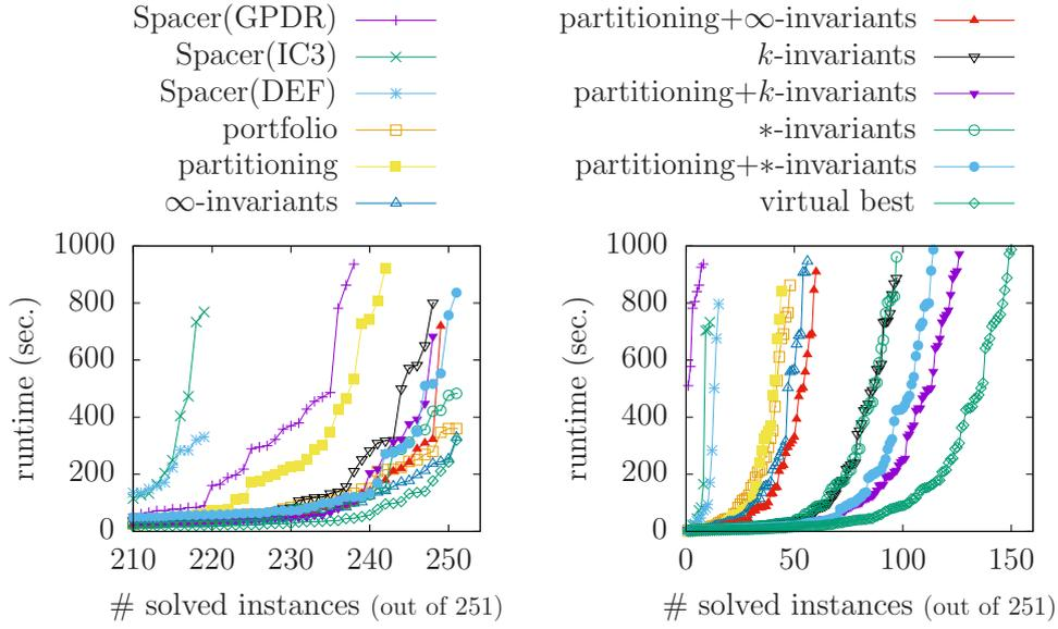
Figure 4.1. Comparison among all the considered techniques on the sets less500 (left) and more500 (right).  $k$ -invariants refers to sharing only lemmas from the trace,  $\infty$ -invariants refers to sharing just  $F_\infty$ , while  $*$ -invariants implements both. Finally, for each benchmark the virtual best runtime among all the tested techniques is reported.
