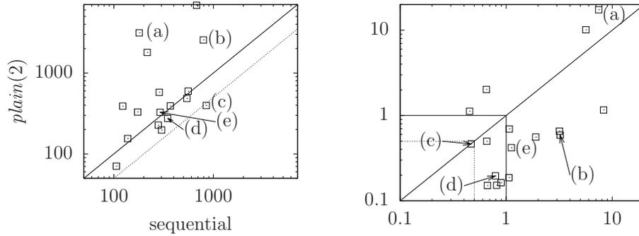
Figure 3.6. Comparison of OpenSMT2 and *plain* for QF\_UF benchmarks (left), and relative run times of the partitions with respect to the original instance (right). The dotted line represents linear two-fold speed-up, and the labels (a) – (d) refer to instances that are analyzed in fig. 3.7 more in detail. The instance (e) is analyzed separately in fig. 3.8 (right).
