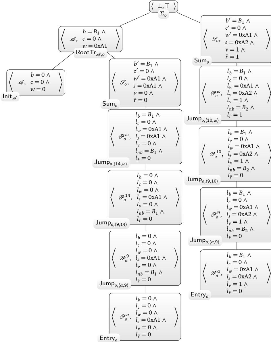
Figure 6.3. A refutation tree for the set of CHCs shown in fig. 6.2 modelling the contract **Auction** shown in fig. 6.1.  $\Sigma_o$  is the CHC  $\mathcal{A} \wedge \mathcal{S}_o \wedge \tilde{r} \implies \perp$ .  $B_1 = 2^{256} - 5 \times 10^{15}$ , and  $B_2 = 2^{256} - 5 \times 10^{15} + 1$ . The values `0xA1` and `0xA2` represent two ETHEREUM addresses.
