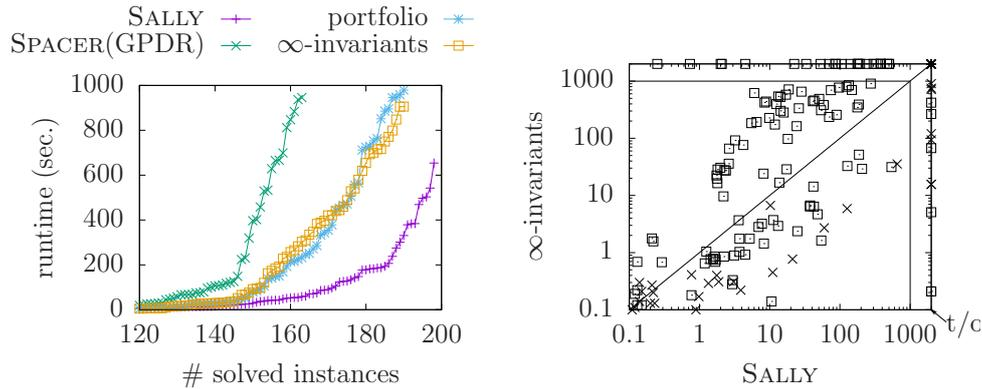
Figure 4.6. On the left, the comparison between sequential Spacer(GPDR) and Sally, and the parallel techniques portfolio and  $\infty$ -invariants using 60 solvers. On the right, the detailed comparison between sequential Sally and  $\infty$ -invariants.
