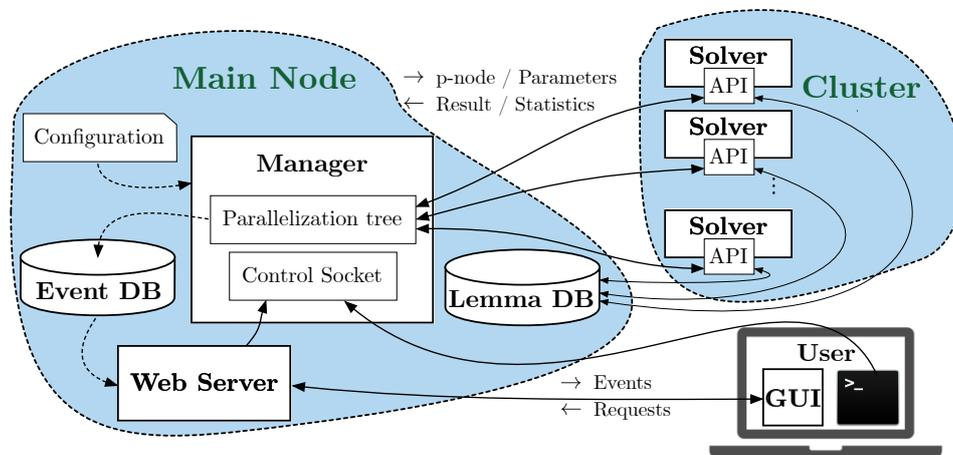
Figure 5.1. SMTS framework overview. Solid lines represent TCP/IP connections, while dashed lines represent disk I/O.
