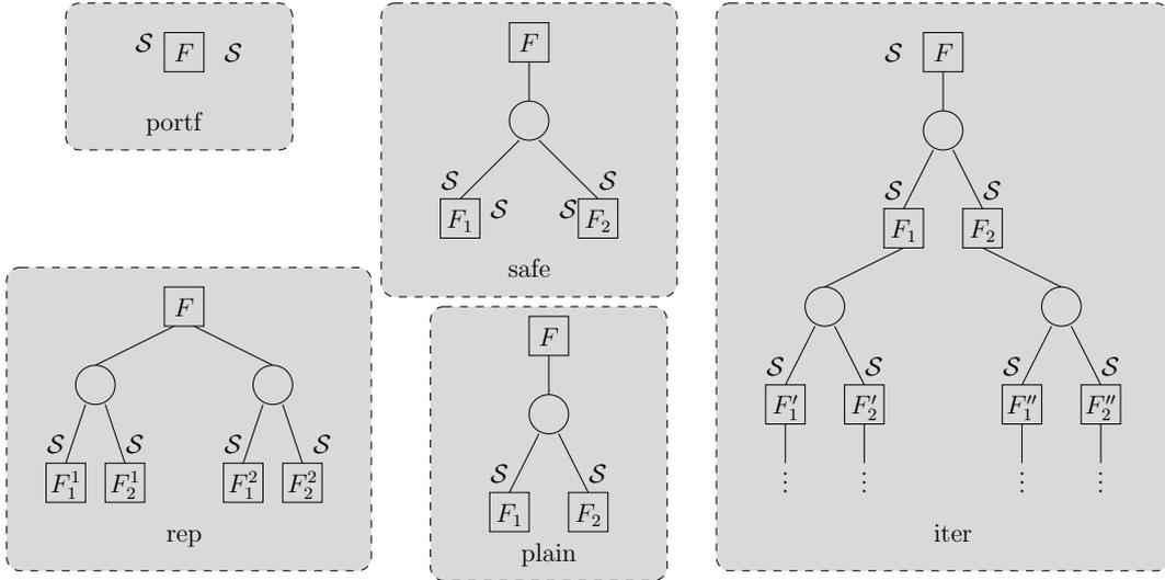
Figure 3.1. Example parallelization trees (clockwise from the top left):  $portf(2, F)$ ,  $safe(2, 2, F)$ ,  $iter(2, F)$ ,  $plain(2, F)$ , and  $rep(2, 2, F)$ . The  $p$ -nodes are drawn with boxes, and the  $r$ -nodes with circles. The SMT solvers are indicated with the symbol  $\mathcal{S}$ .
