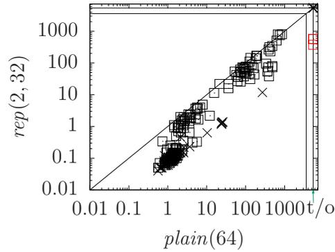
Figure 3.10. The run times for the parallelization algorithms  $plain(64)$  and  $rep(2, 32)$  on 64 cores.
