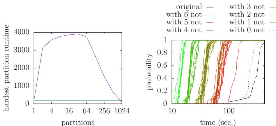
Figure 3.8. Run time with respect to number of partitions for instance (a), green line represent original instance runtime (left), and the cumulative runtime distribution of the QF\_UF benchmark (h) and its 64 partitions (right).
