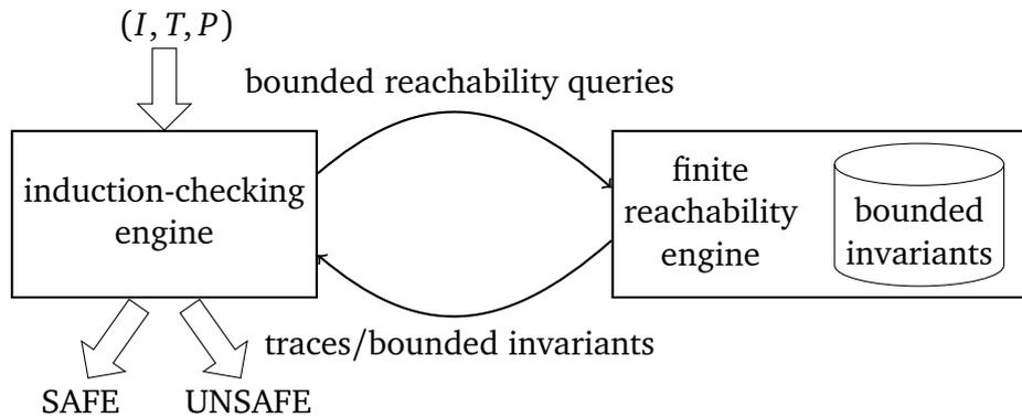
Figure 2.1. The IcE/FiRE framework for solving safety of transition systems
