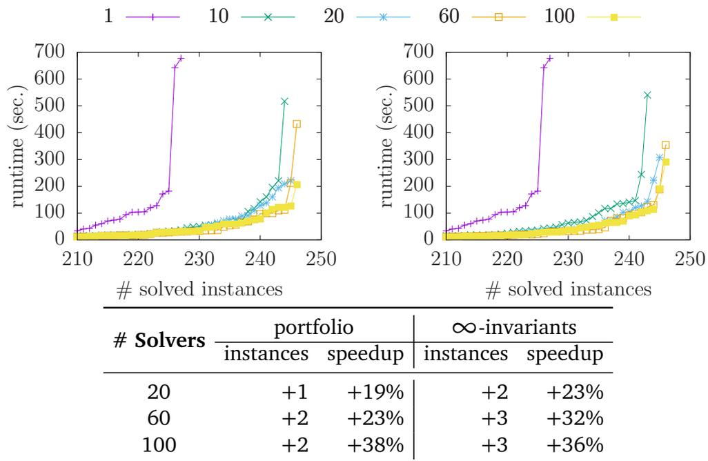
Figure 4.3. Comparison among different degrees of parallelism for portfolio without lemma sharing (left), and portfolio with  $\infty$ -invariants sharing (right) on less500. The table on the bottom reports speedup and more instances solved compared to 10 solvers.
