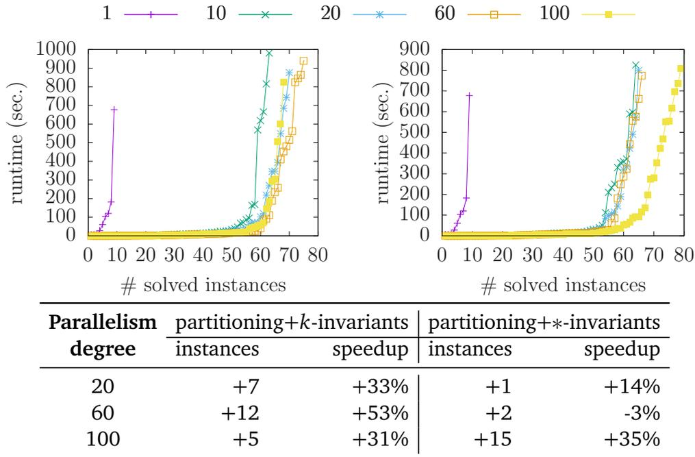
Figure 4.4. Comparison among different degrees of parallelism for partitioning with  $k$ -invariants sharing (left), and partitioning with  $*$ -invariants sharing (right) on more500. The table on the bottom reports speedup and more instances solved compared to 10 solvers.
